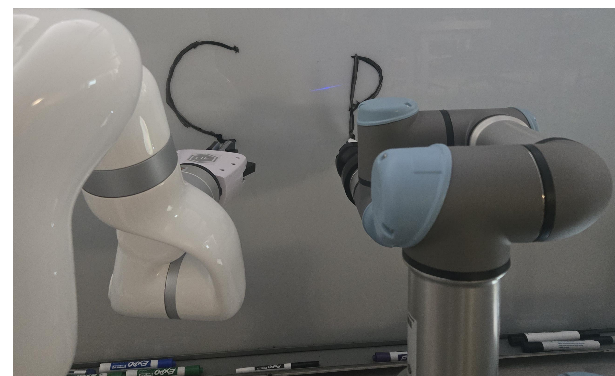
Fig. 5: UR3e and xArm 5 cobots write by following mouse front view
